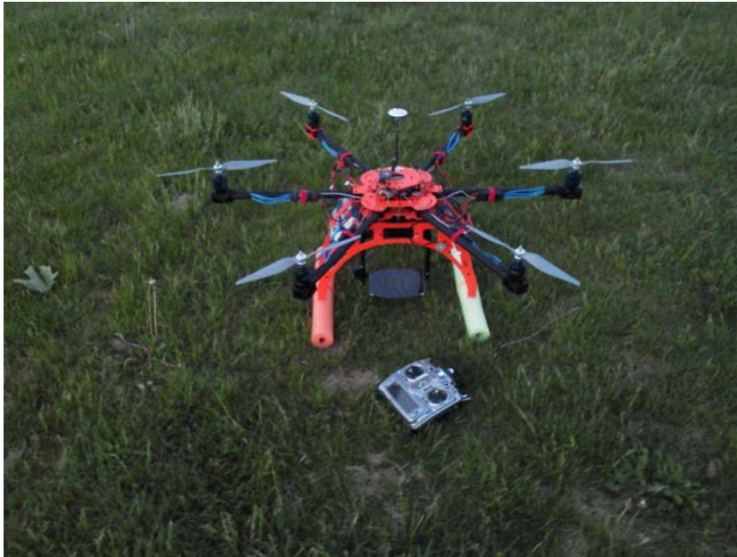
Figure 1: A Bergen hexacopter recently acquired by the project team as part of a demonstration of the capabilities of multi-rotor remote control helicopters. The system is capable of deploying the same Nikon D800 digital camera as sensor as the Bergen Tazer 800 single-rotor platform but is significantly simpler and easier to fly.
