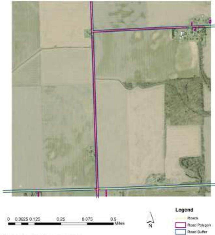
**Figure 11. A "no-trees over roads" example image that will be the beginning basis of the ROC curves for detection and classification of unpaved roads under ideal conditions, improving the accuracy of the thresholds used to map the unpaved roads in eCognition. The purple areas are the polygons from eCognition, the blue is the 30-foot Michigan Framework Roads Network buffer.**
