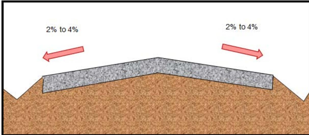
**Figure 2: Road cross section illustrating an example of a typical cross slope.**
